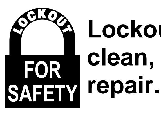
Lockout power to clean, oil or repair.
